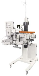
The overall material is carbon steel, which is suitable for applications in various industries. Movable casters are convenient to move the equipment, and the base is strengthened to ensure the stability of the equipment. The whole plate is cut and welded, with beautiful appearance and reliable quality.
